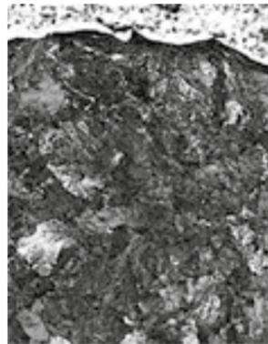
A micrographic study of the braze weld of the plate to the rail shows that the steel structure in the rail remains unchanged, totally pearlitic and with no cracks.
