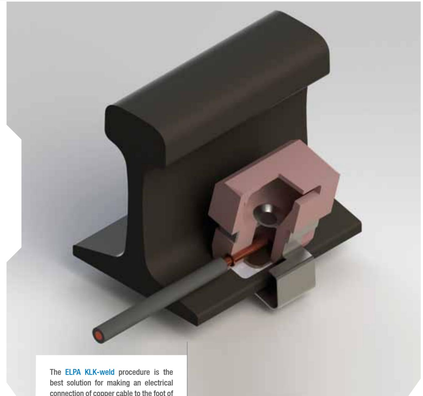
The ELPA KLK-weld procedure is the best solution for making an electrical connection of copper cable to the foot of the rail, since a low electrical resistivity and a high mechanical strength are achieved in the connection without affecting the rail steel, because its temperature never exceeds 500°C.
