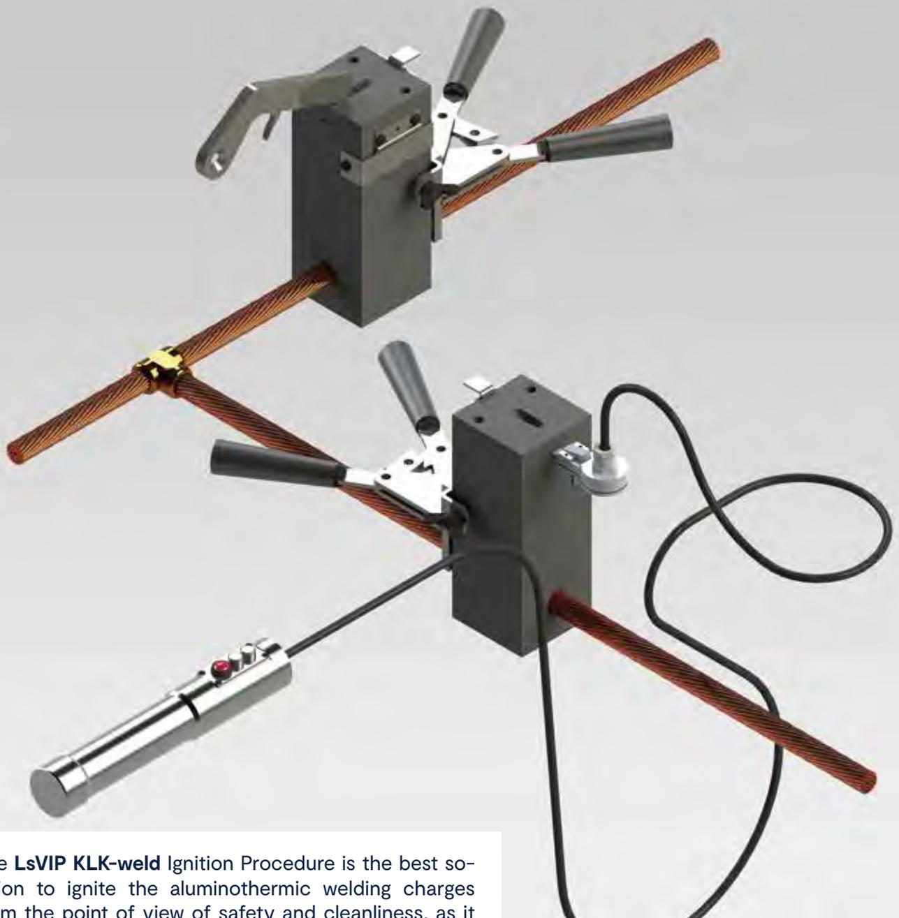
The **LsVIP KLK-weld** Ignition Procedure is the best solution to ignite the aluminothermic welding charges from the point of view of safety and cleanliness, as it prevents spattering from the crucible-mould during the aluminothermic reaction, minimizes smoke emissions and, furthermore, it enables the charge to be ignited at a certain distance from the mould, using the **KLK-weld Remote Ignition Device**.
