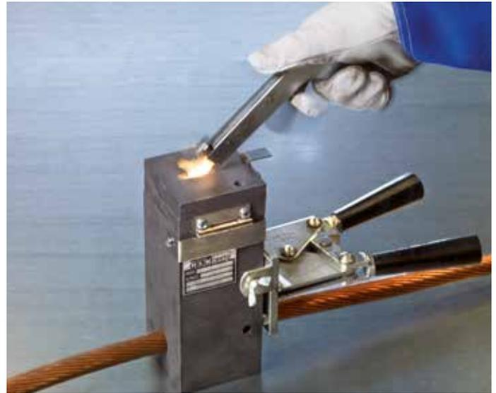
The **LsVIP KLK-weld Ignition Procedure** uses a special lid that completely closes the mould crucible, so that it prevents spattering from the aluminothermic reaction. But at the same time it allows the release of overpressures within the crucible. Furthermore, the smoke emissions are much lower than in other ignition procedures.
