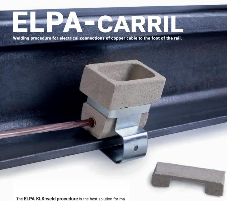
king electrical connection of copper cable to the foot of the rail, since a low electrical resistivity and a high mechanical strength are achieved in the connection without affecting the rail steel, because its temperature never exceeds 6000C.
