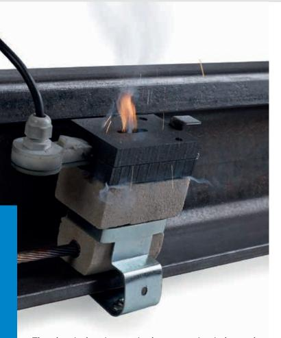
The electrical resistance in the connection is lower than 10-5  $\Omega$ , and the mechanical shear strength in the rail/plate joint is greater than 50 kN.
