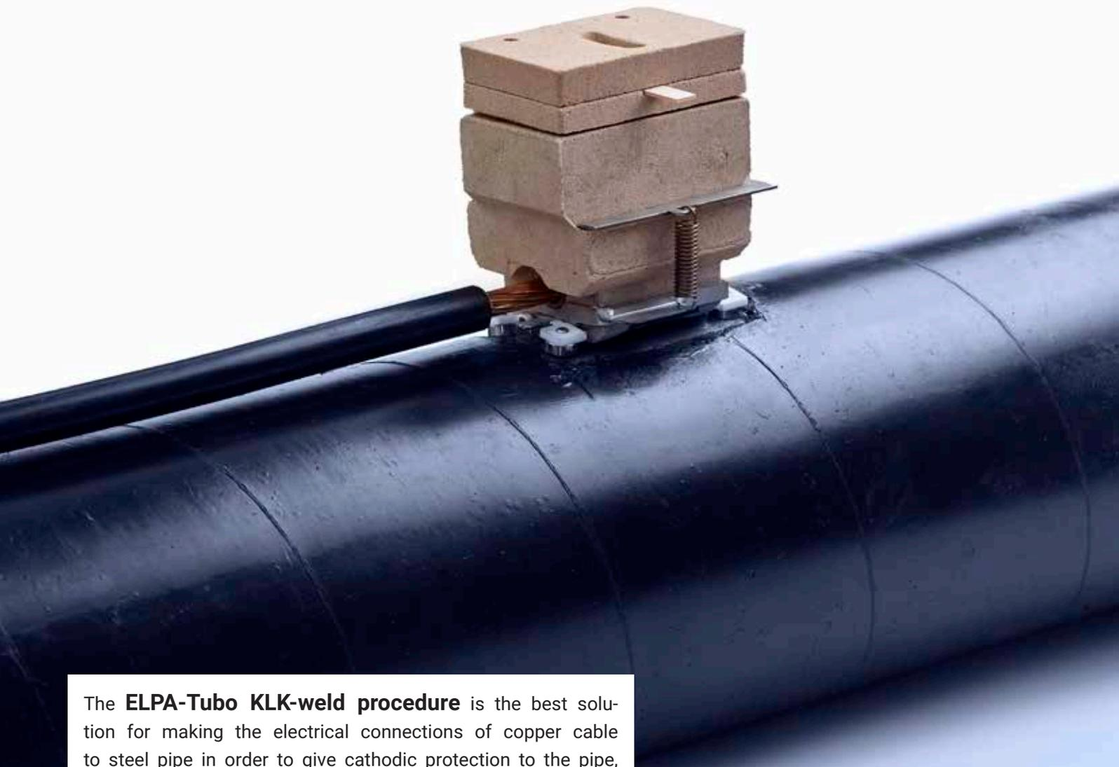
The **ELPA-Tubo KLK-weld procedure** is the best solution for making the electrical connections of copper cable to steel pipe in order to give cathodic protection to the pipe, as the resulting weld has a low electrical resistivity and a high mechanical strength in the connection. **This procedure does not change the structure of the steel pipe** as the temperature never exceeds 450°C.
