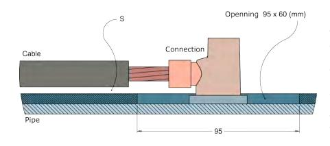
The area to be protected includes the opening made in the insulation of the pipe, of dimensions  $95 \times 60$  (mm), the end of the cable whose insulation had been removed in a length of 50 mm, and the connection itself. The space between cable and pipe insulation (S) favors the flow of the coating resin in that area.
