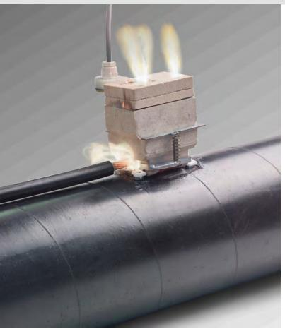
As the mechanism that attaches the mould to the pipe does not include any embracing element, the pipe does not need to be completely unearth; it is sufficient to uncover the top of the pipe.
