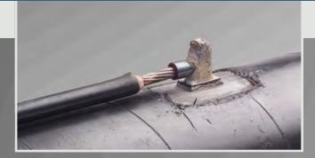
The **ELPA-Tubo KLK-weld** procedure is the best solution for making the electrical connections of copper cable to steel pipe in order to give cathodic protection to the pipe, as the resulting weld has a low electrical resistivity and a high mechanical strength in the connection. This procedure does not change the structure of the steel pipe as the temperature never exceeds 450 °C.
