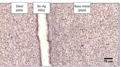
Unlike other welding procedures, the **ELPA-Tubo KLK-weld** procedure does not affect the structure of the steel pipe. A micrograph of the welded joint between the plate and the pipe reveals that the structure of the steel pipe remains unchanged and free from micro-cracks.
