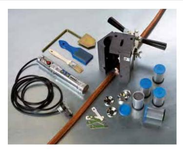
The **KLK-weld Remote Ignition Device** includes sufficient cable to allow the charge to be ignited at a certain distance from the mould where the reaction takes place. It only requires two standard batteries and it includes warning lights that indicate when the batteries are dead or if the fuse is properly inserted into the clamp.
