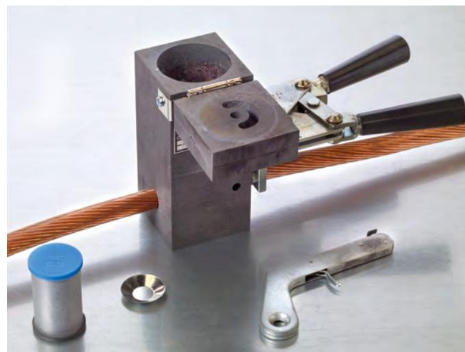
The **KLK-weld Remote Ignition Device** includes sufficient cable to allow the charge to be ignited at a certain distance from the mould where the reaction takes place. It only requires two standard batteries and it includes warning lights that indicate when the batteries are dead or if the fuse is properly inserted into the clamp.
