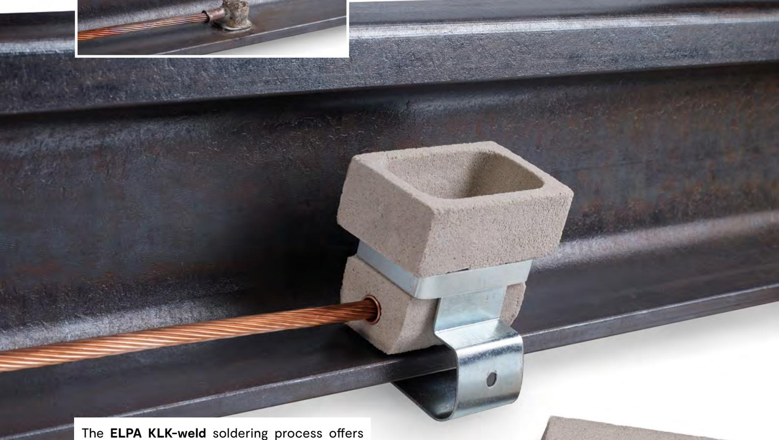
The **ELPA KLK-weld** soldering process offers the best solution for soldering copper cables to the rail base. The result is a connection with a very low electrical resistivity and a high mechanical resistance without modifying the steel of the rail because its temperature never exceeds 600 °C.
