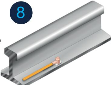
**IMPORTANT NOTE:** If traffic passes within one minute after ignition, the welding must be removed and repeated. It can be done in the same place, without risk to the rail, after the rail cleaning operations have been carried out again.
